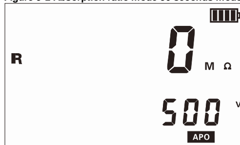
Figure 9-4 Insulation resistance measurement mode
