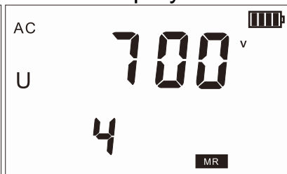
Figure 13-2 AC voltage check
