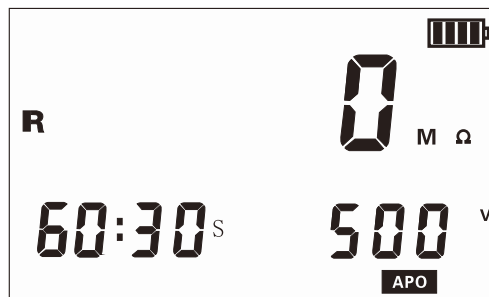
Figure 9-2 Absorption ratio mode 30 seconds mode
