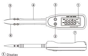
(2) "(a) " Button: holds current reading on screen
