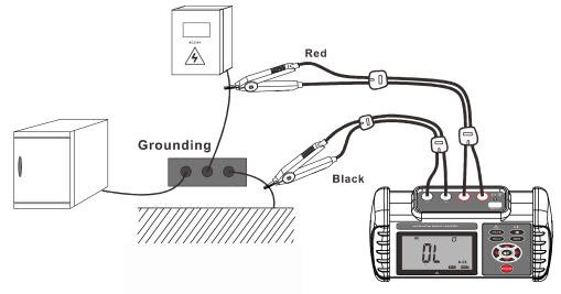
The following figure shows an example to test the resistance value of two metal connectors.
