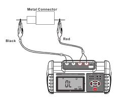
The following figure shows an example to test the resistance value of the contact point of the relay.
